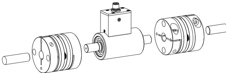
Illustration 7: assembly of the clamping hubs
