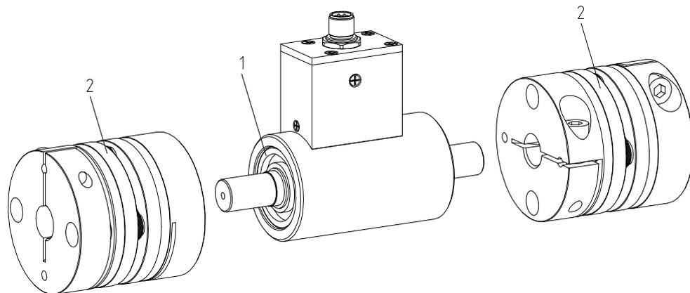
Illustration 3: DATAFLEX® 16 - torque measuring shaft with RADEX®-NC
