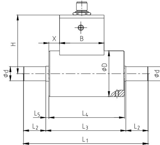
Illustration 1: DATAFLEX® torque measuring shaft
