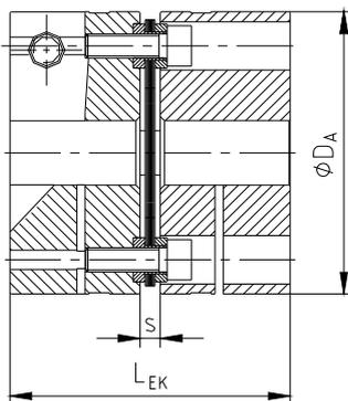
Illustration 9: assembly of the coupling
