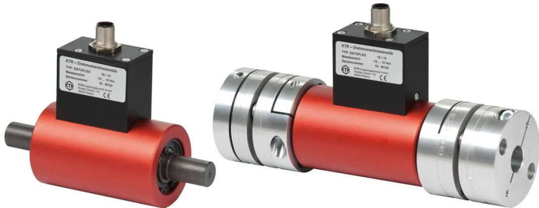
**DATAFLEX®** is a maintenance-free torque measuring shaft with integrated speed measurement. Combined with the steel lamina coupling **RADEX®-NC** the complete system forms a torsionally stiff, double-cardanic coupling with integrated measuring shaft.
